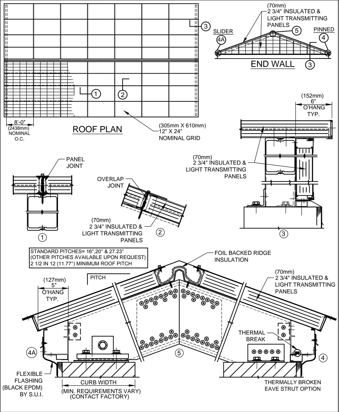
**CENTER RIDGE SKYLIGHT W/ MINIMAL OUTWARD THRUST DESIGN**
